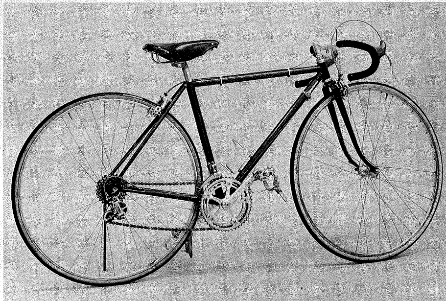
Hugh Enochs: This 18-inch frame, built for a woman who is just five feet tall and has short legs, still uses 27-inch wheels. The frame features lugless construction and a sloping top tube. (C. Russell Wood photo)
